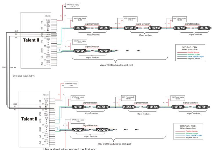
Use a short wire connect the first port, and connect with the black wire of module, then connect to the negative of the power supply
