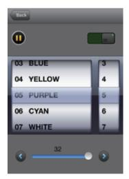
5. In the middle part, slide to select different lighting effects. and slide the number in the right side to change the speed.
