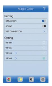
2. Open the "Simulation" and close the "Sound" function, and click the "WF300 >" button enter the "SPI setting page".
