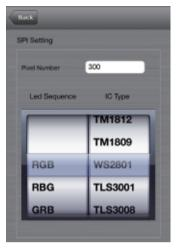
3.Select the "RGB" as the value of Led Sequence and set the IC Type to be WS2801. Then set the value of "Pixel Number" according to the quantity of TriCo RGB modules in your project.
